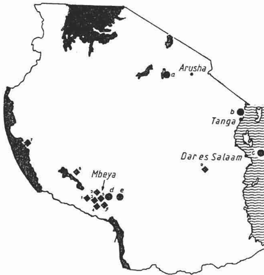
Fig. 1 - Sketch map of Tanzania, showing the locations of principal phosphate deposits. Black squares: carbonatites; black circles: phosphorites. Numbers and letters indicate the following localities: 1: Musensi, Mbeya region; 2: Songwe Scarp, Mbeya region; 3: Sukomaweru, Mbeya region; 4: Sageri Hill, Mbeya region; 5: Mballizi, Mbeya region; 6: Panda Hills, Mbeya region; 7: Sangu Ikola, Rukwa region; 8: Ngualla, Mbeya region; 9: Zizi near Kisaki, Morogoro region; a: Minjingu, Arusha region; b: Amboni caves, Tanga region; c: Latham island, 60 km east of Dar es Sallam (compiled after different sources).
