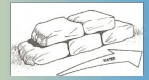
Sandbags should be placed in staggered layers or heap in pyramids (see diagrams).
