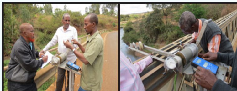
Discharge measurement at a bridge in Lower Thiba River, Embu
